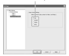
After you change the colour system settings and close the [Video Settings] screen, the NetAV connection will be disconnected and then it will be reconnected automatically.
